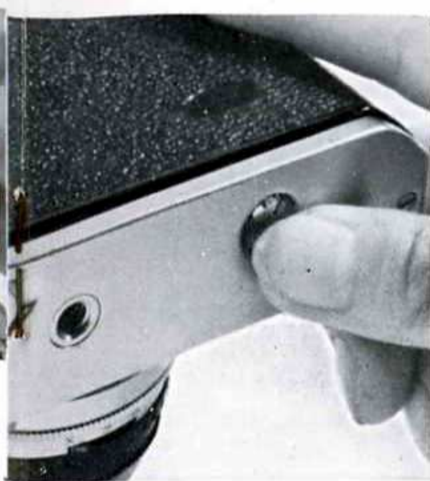
(2) Combine a red spot on the hood with another red spot on the lens ring.
