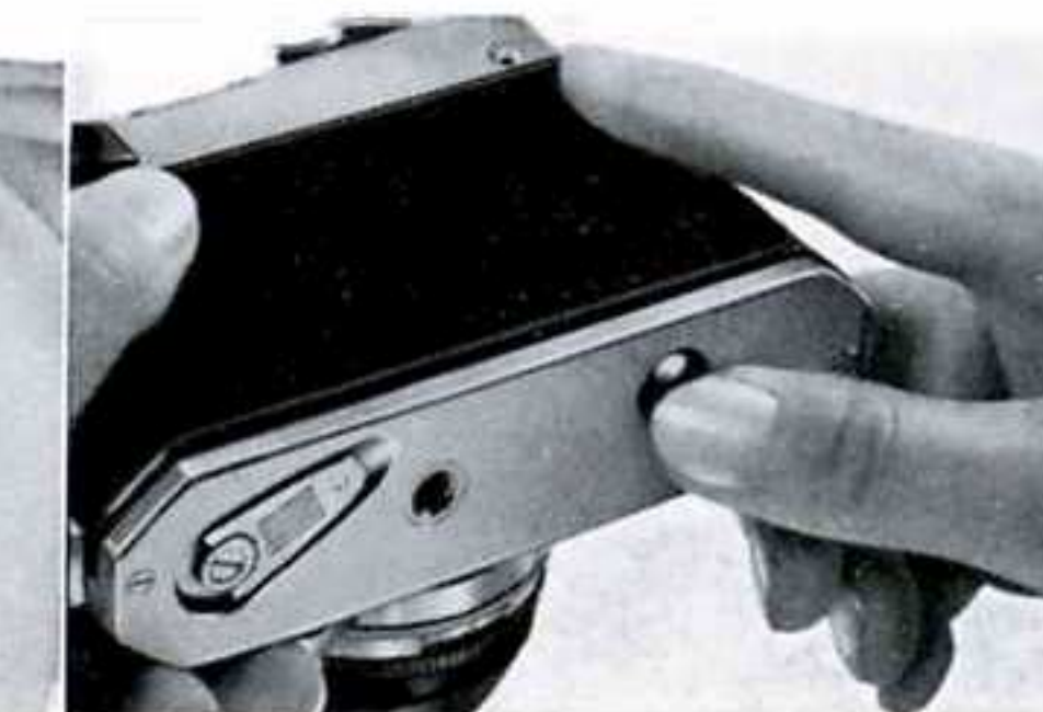
10. When all of the film has been exposed, push Rewind button.
