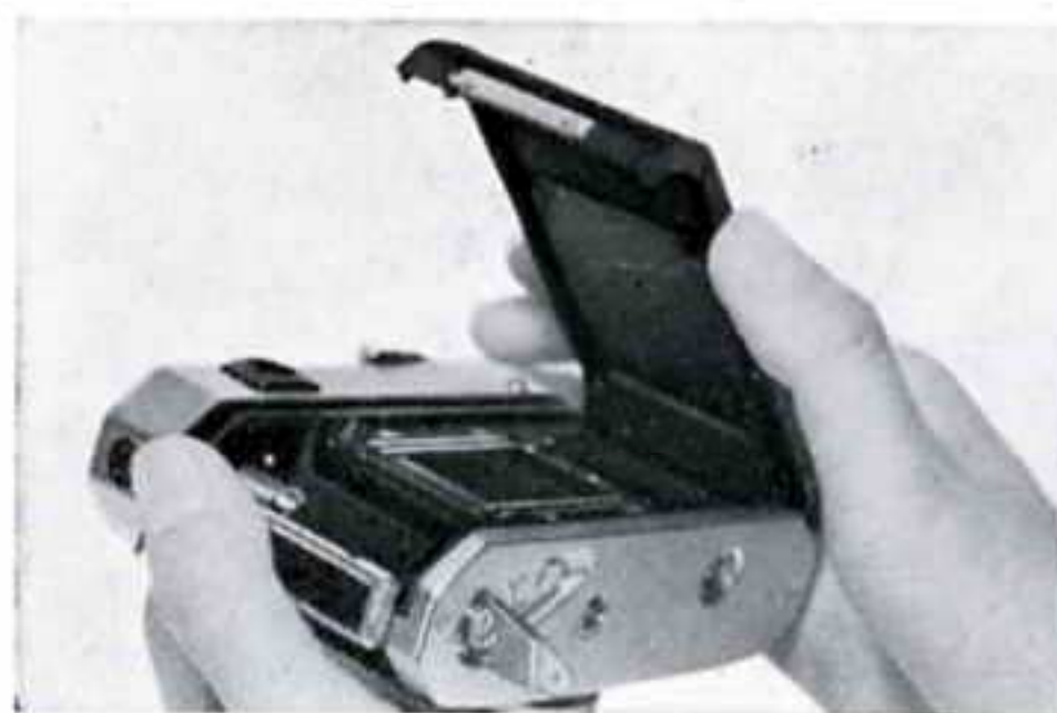
1. Turn Back Lock Key in the direction of "0".
