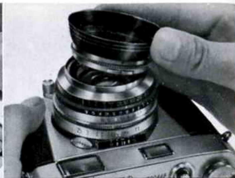
(2) Combine a red spot on the hood with another red spot on the lens ring.
