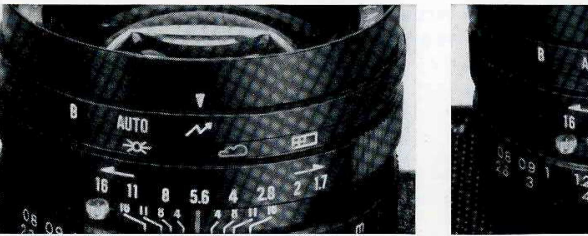
Set the flash mark  $\checkmark$  to the index line by turning the Exposure Control Ring. The shutter speed is set automatically at 1/30 sec. Electronic flash or flashbulbs can be used as the shutter speed is set at the X setting.
