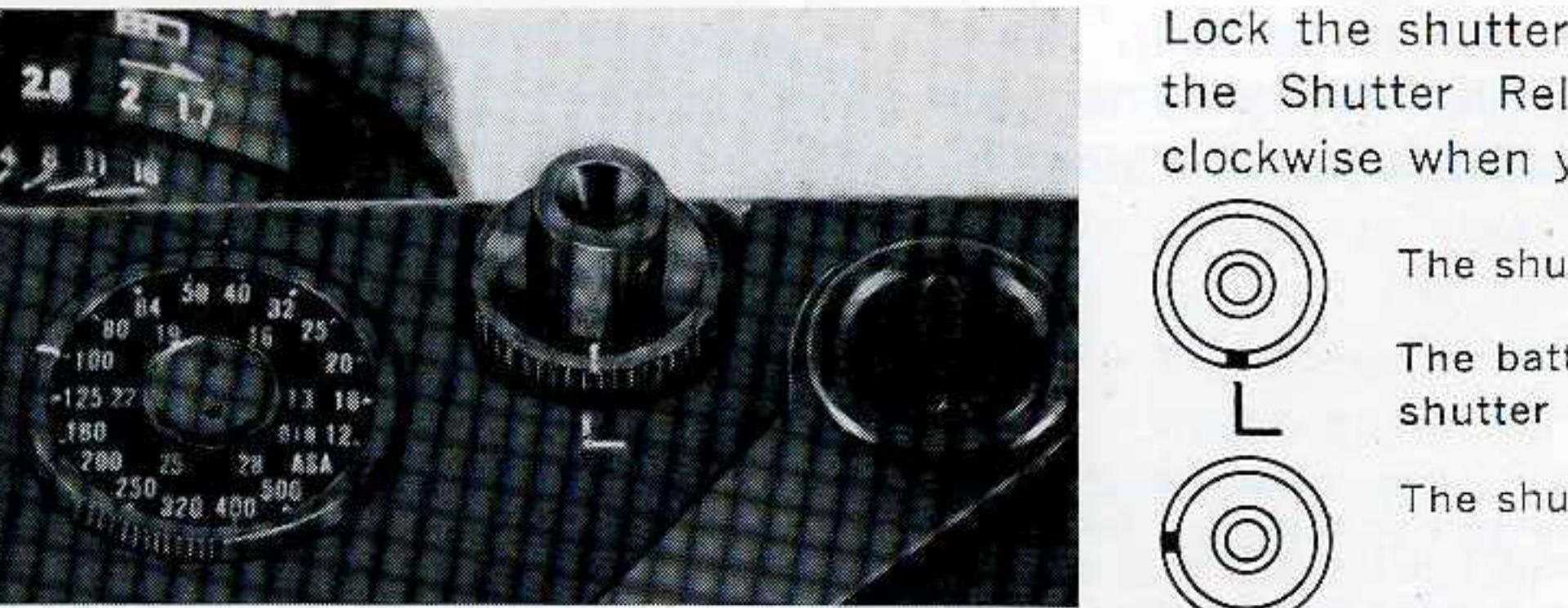
Lock the shutter release button by turning the Shutter Release Lock Ring counter-clockwise when your camera is not in use.
